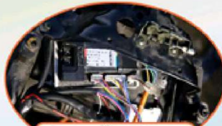
Controller Wiring harness
